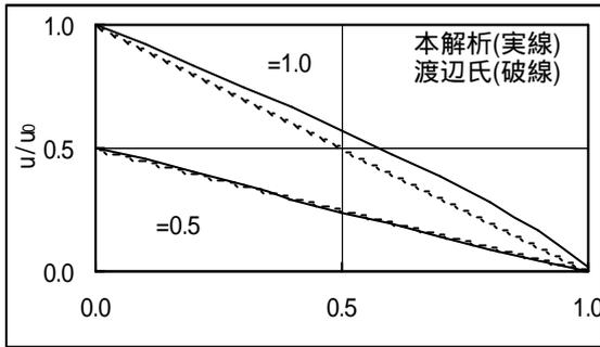
図-5 端面摩擦のuに与える影響 (  $\alpha=0.2, \beta=4, q_0=0$  )
