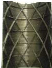
Fig.4 Half Section of Cured Isogrid Cylinder
