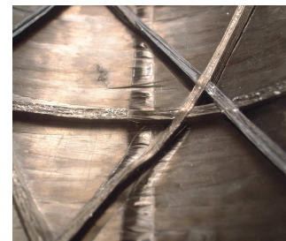
Fig.5 Interior of Isogrid Stiffened Cylinder
