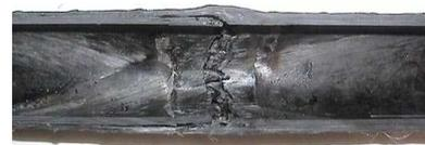
Fig.8 Failure Aspect of the Specimen (100mm, 12Pieces) Cut Section
