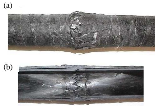
Fig.7 Failure Aspect of the Specimen (100mm, 12Pieces)
