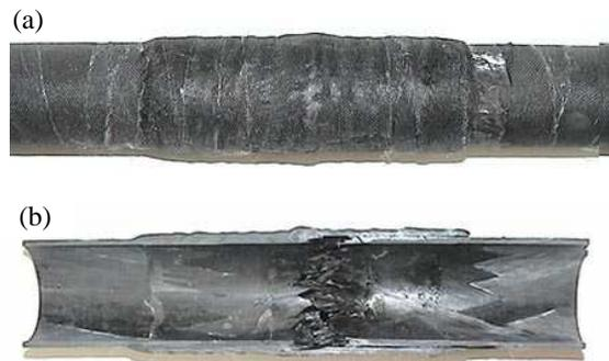
Fig.9 Failure Aspect of the Specimen (50mm, 20Pieces)
