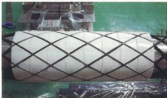
Fig.6 Filament winding process.
