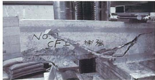
Fig.11 Failure aspect after bending test (No.4-1).
