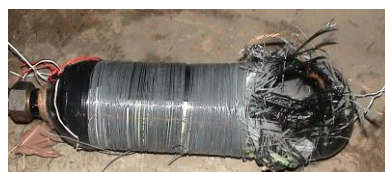
Fig.3 Specimen after Burst (Compressive Strain 2%)
