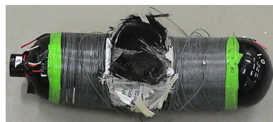
Fig.2 Specimen after Burst (Compressive Strain 0.5%)
