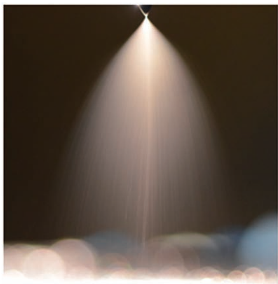
Fig.1 Magnified photo of electrostatic spray
