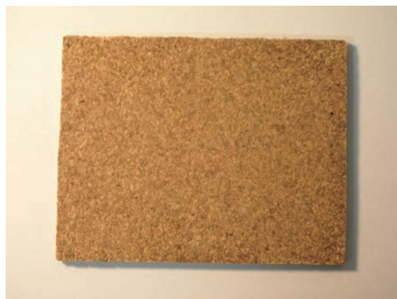
Particle board using peanut husks and PVA
