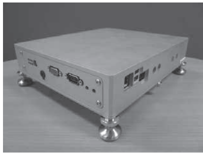
Fig. 6 Track condition monitoring system using in-service vehicle
