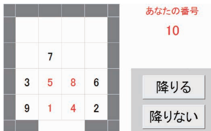
Fig. 10 Screen of the guidance system (The red numbers in the elevator show persons getting off.)
