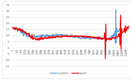
Fig.18 joint torque and muscle torque of shoulder elevation right with J turn. Blue for joint torque and red for muscle torque.
