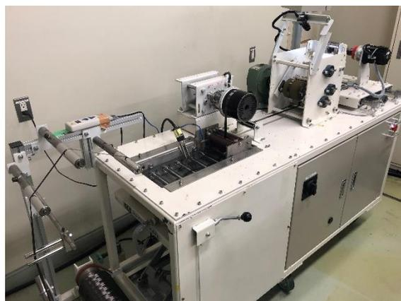
Fig.1 Fiber opening machine
