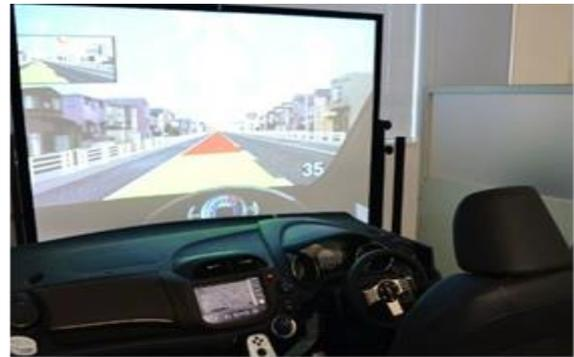
Fig. 5 Overview of fixed-base driving simulator
