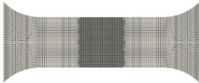
Fig.4 Mesh of tensile test specimen model
