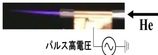
Fig.1 Atmospheric pressure Helium plasma jet
