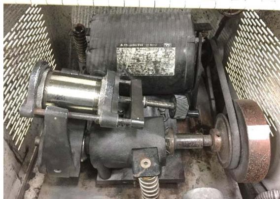
Fig. 3 Vibratory ball mill (SPEX 8000 Mixer/Mills).
