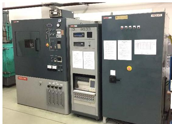
Fig. 4 SPS system (DR.SINTER SPS-1050).
