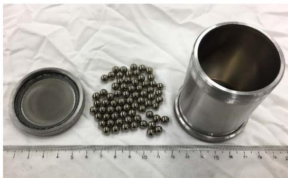
Fig. 2 Tool steel vessel and tool steel balls.
