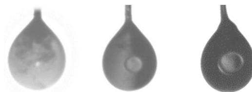
(a)Internal cloud (b)Secondary droplet (c)Secondary droplet (OME/methanol (OME/methanol (OME/ethanol/water droplet) droplet) droplet)
