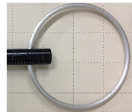
Fig. 9 Loop antenna (MK-5S) used for receiving radio wave
