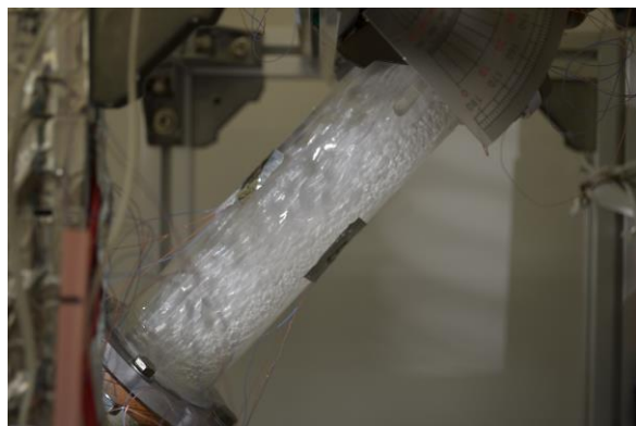
Fig.5 Flow inside of the heat pipe. (diameter 34mm,potassium oleate 100ppm)
