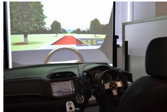
Fig. 2 Overview of fixed-base driving simulator
