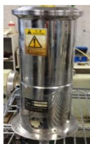
Fig.3 Resin tank
