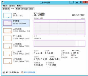
Fig. 25 Memory utilizations under standby with four virtual machines
