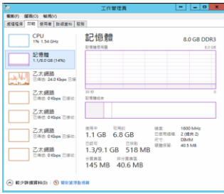
Fig. 14 Memory utilizations under standby without virtual machine
