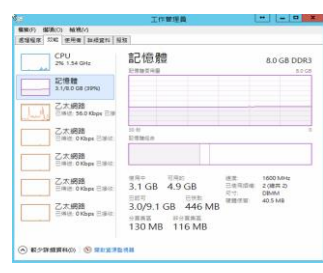
Fig. 19 Memory utilizations under standby with two virtual machines
