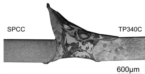
Fig.3 Macrostructure of welded joint. (Flange TP340C, V=1002mm/min)
