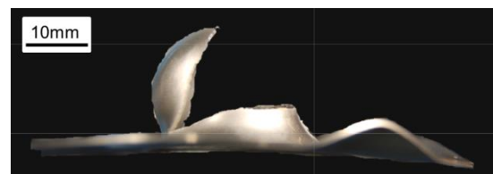
Fig.7 Appearance of erichsen tested specimen.
