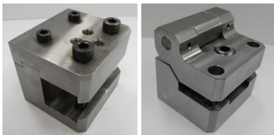
Fig.6 The difference in the bolt number of chuck
