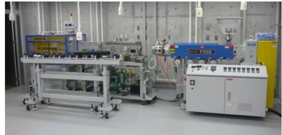
Fig.6 Extrusion molding machine
