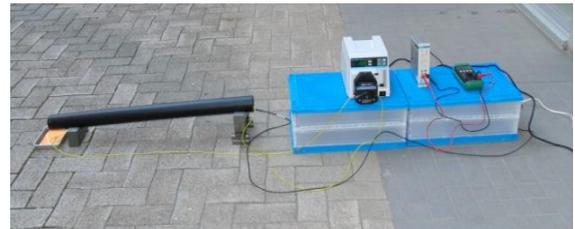
Fig7 Experimental apparatus for sensor evaluation with double tube
