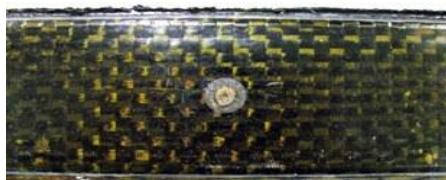
Fig.2 Surface of specimen with resole coating
