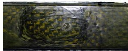
Fig.1 Surface of specimen without resole coating
