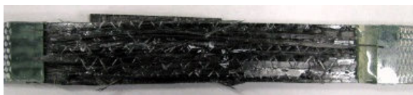
Fig.13 Fracture surfaces of ripoxy
