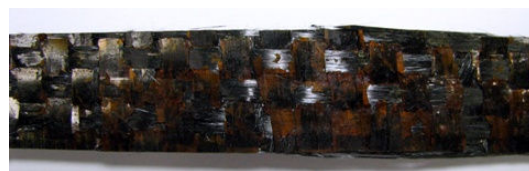
Fig.6 Fracture surfaces of conventional resin
