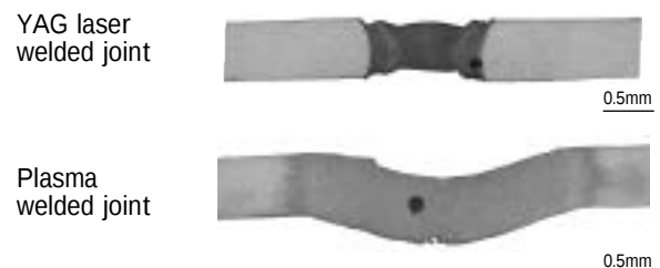
Fig.6 Macrostructures of welded joints. (AZ61)
