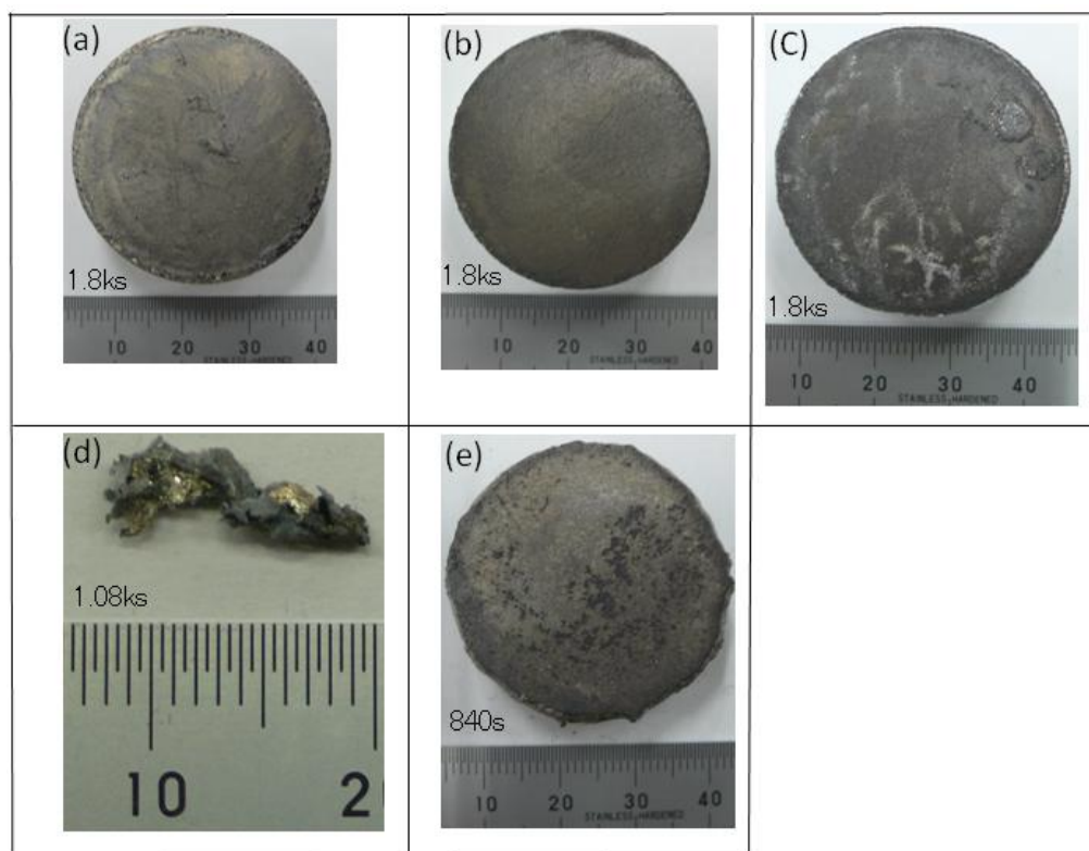
Fig4 Surfaces of Mg-1 mass%TiH 2 fabricated from cold compacted precursors with different holding temperatures (a)673K,(b)723K,(c)773K,(d)823K and (e)873K
