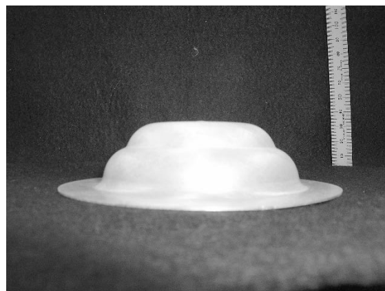
Fig.9 Blown cups from sheet annealed at 573K, Blowing at 623K for 2100sec
