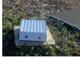
Fig.2 Outside Appearance of measurement system      Fig.3 Flat Array Sodar and Enclosure
