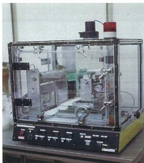
Fig.2 Electro spinning machine
